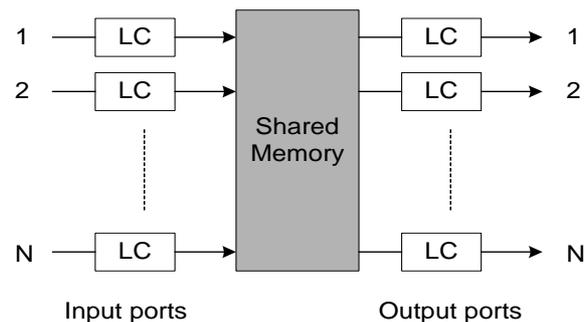
**Figure 1:** Shared memory switch architecture
