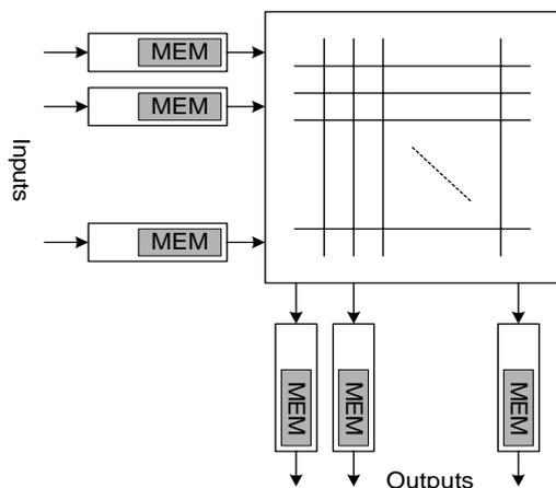
**Figure 3:** Crossbar based switch
