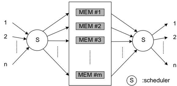
**Figure 7:** Parallel memories shared by all the inputs
