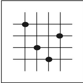
**Figure 4:** A configuration of a 4x4 crossbar switching fabric
