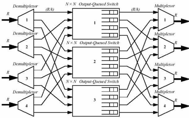
**Figure 9:** Parallel Packet Switch
