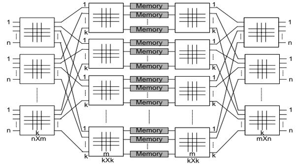
**Figure 12:** Central Buffered Clos-network switch
